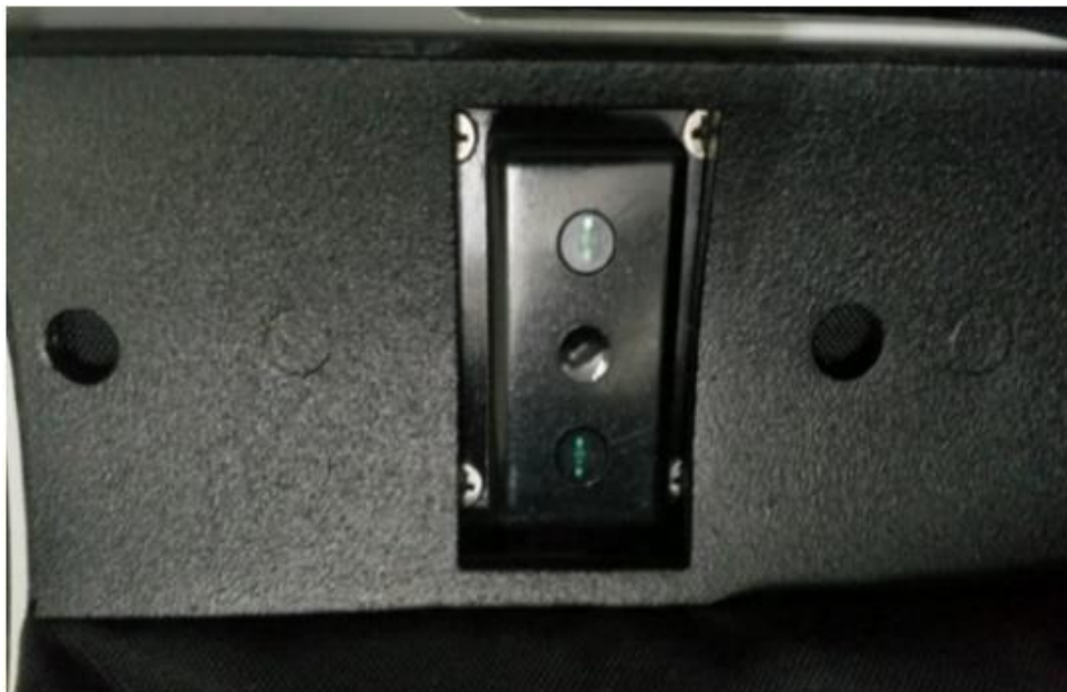
Figure 2: NIR device used to measure the body fat.
