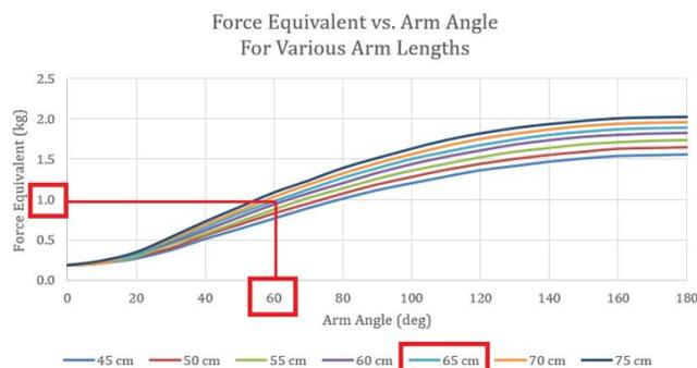
**Figure 8:** An example scenario illustrating the use of Figure 5. Here, a patient’s arm is 65 cm in length, and the arm angle is 60°, resulting in a force equivalent of 1.0 kg.
