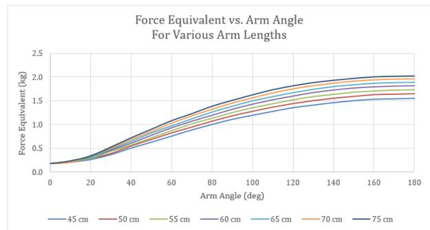
**Figure 5:** Lookup chart showing the TheraBand kg equivalent force as a function of arm angle for various arm lengths.
