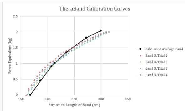
**Figure 2:** Calibration curve showing kg-equivalent force vs. stretched length of Band 3, later used by volunteers, along with that for the calculated average of all eleven bands, excerpted from Figure 1 for comparison. The black curve is a guide for the eye.
