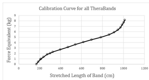
**Figure 1:** Calibration curve for the average of all eleven TheraBands. The black curve is a guide for the eye.
