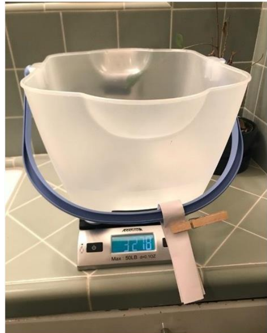
Figure 4: Recording the threshold weight of the bucket of water - i.e., the maximum weight before slippage occurs.
