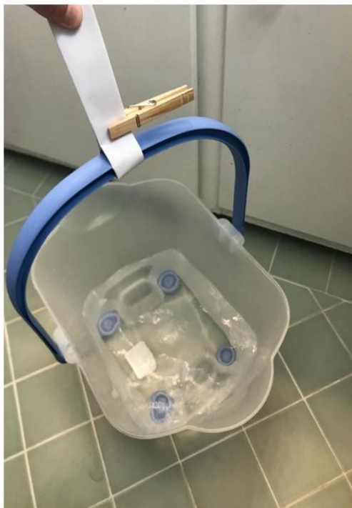
Figure 3: Apparatus including 2.5 gallon bucket, water, clothespin, and copy paper.
