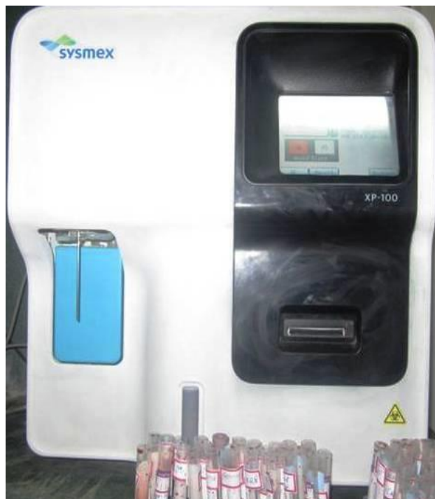
Figure 2: Sysmex XP 100 for evaluation of complete blood picture including the platelet counts.
