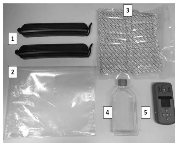
Figure 1: Items that compose the hypoxia chamber; 1: Clips used to seal; 2: Plastic bag; 3: O 2 absorbers; 4: Cell culture flask; 5: O 2 sensor.
